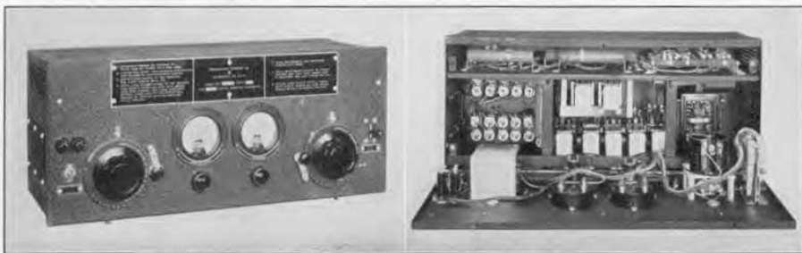
Figure 17. Panel and interior views of the air-brake test set. The dials control identical rheostats, one of which can be seen at the right in the interior view, ganged with another, smaller, rheostat.
