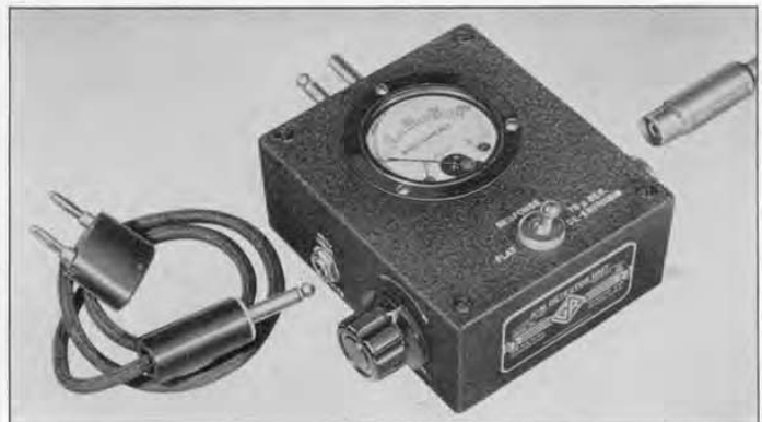
Figure 4. Close-up view of the A-M Detector Unit. The coaxial connector at the right is supplied with the unit; the cord, plug and jack at the left are not.
