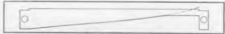
Figure 15. Mandrel shape used for the "C"-bias rheostat in the tube checker of Figure 16.
